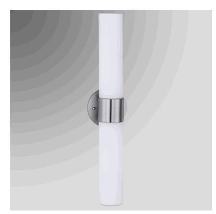
24"H Brushed Nickel 2-Light Wall Sconce, two GU24 sockets, Direct Wired with Opal Glass Diffusers. Recommend two 8 watt PL or 11 Watt LED PL bulbs with GU24 base.
